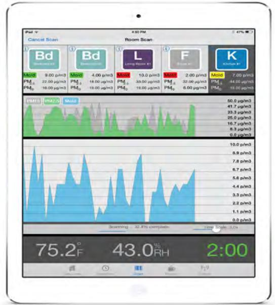
**The MouldScope is the only instrument in the world that extends differentiation to bioaerosol classes - fungi, pollen and bacteria - as well as particulate matter, in one operational unit.**
